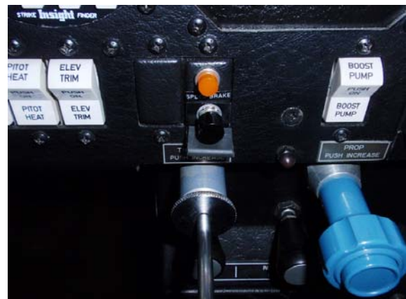
New guard just below black speed brake switch
